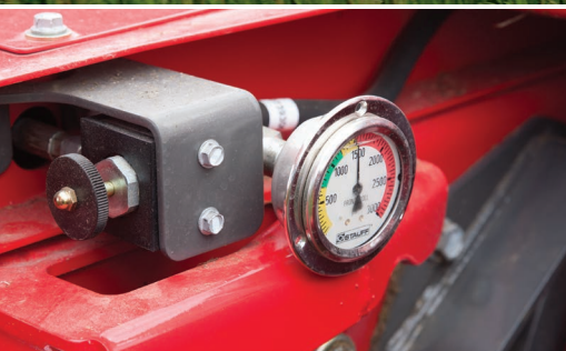
Hydraulic conditioning roll tension on the 1393 & 1316S. This is the first pull-type design to have this system.
