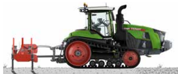
Figure 1: A tractor goes to work without proper tractor and implement weight distribution. This results in insufficient front weight on the tractor, and as a result increases slip.
