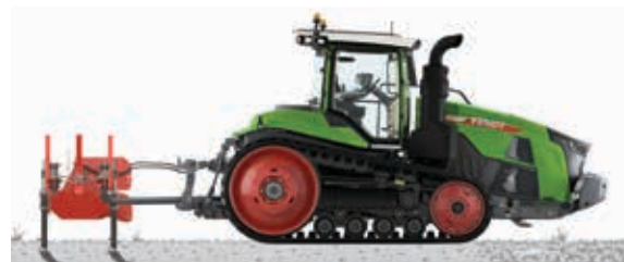
Figure 2: The 1100 Vario MT with Smart Ride Plus allows for easy adjustment of the weight distribution. This results in reduced slip, improved ride comfort, and improved overall performance.
