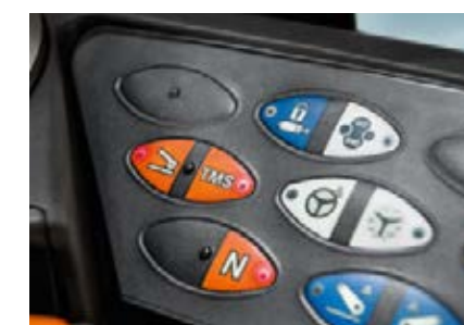
All functions are arranged simply and straightforward on the backlit membrane keypad according to the tried and tested Fendt operating logic.
