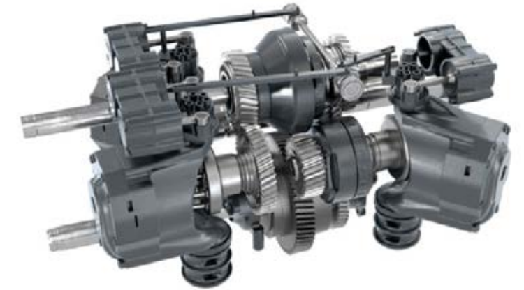
New, larger high-capacity hydrostats with 370 cm 3 ensure very high transmission efficiency. The separate oil supply protects the gearbox against oil mixing and contamination.
